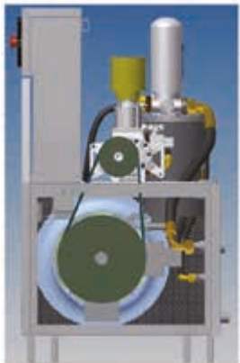
Belt Auto Tensioning system
